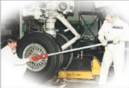
An EDS Dial Measuring Wrench being used on the Nose Wheel bearing assembly of a Boeing 747-436 aircraft.
