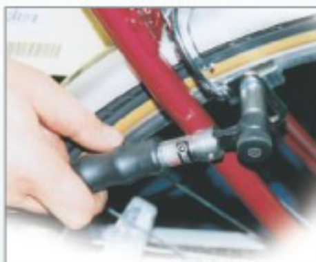
A TBN 10 'Breaking' Torque Handle being used to assemble bicycle brake shoes at Raleigh Industries.
